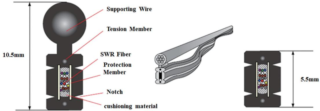
Fig. 8. 24-fiber aerial distribution optical cables <sup>5)</sup>.
