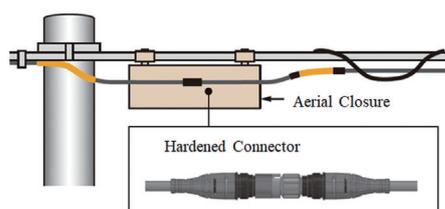
Fig. 2(a). Example deployment for replacement of the closures.
