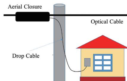
Fig. 1. Schematic of cable wiring.
