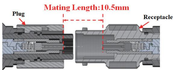
Fig. 6(a). Mating length of hardened connector.
