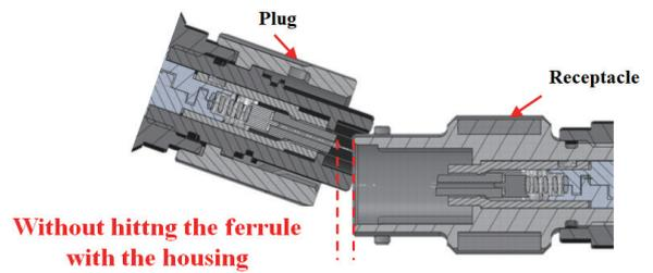
Fig. 6(b). Designed to prevent interferences between the ferrule and the housing.
