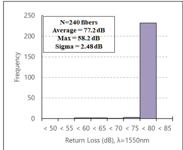
Fig. 11(b). Return loss of hardened connector at 1550nm.
