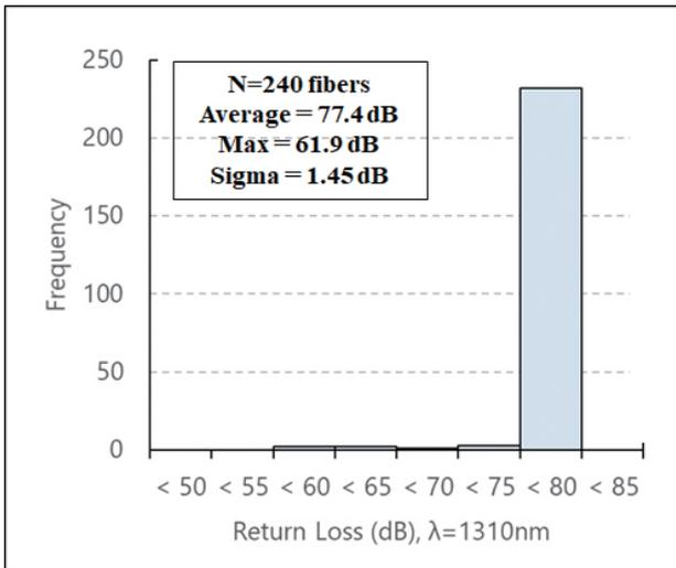
Fig. 11(a). Return loss of hardened connector at 1310nm.
