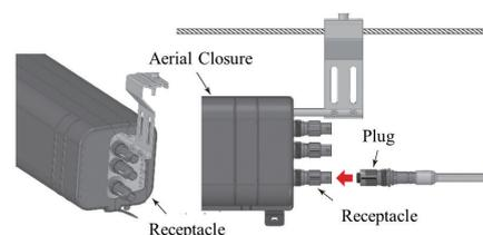
Fig. 2(b). Example deployment of hardened connector onto the closures.
