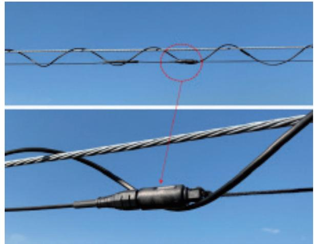
Fig. 9(b). Connector pulling.
