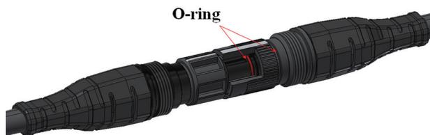
Fig. 7. Sealing structure.
